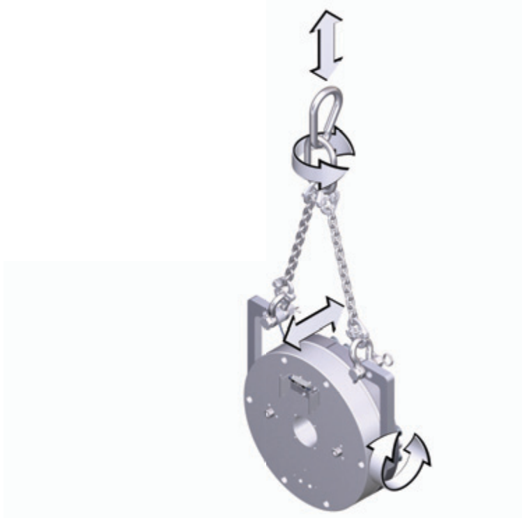
Fig. 8: Lifting mechanism for hooking onto a hoist
